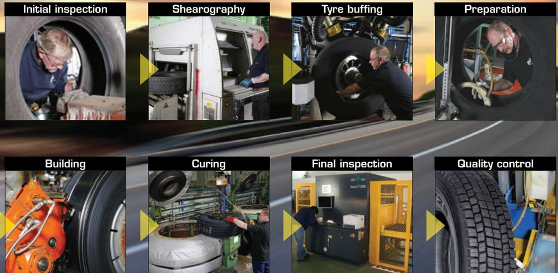
The Lodge Retreading Process involves taking a worn casing of good structure and quality and completely renewing the tread and the sidewall rubber. The rebuilt tyre then goes through a curing process during which the new rubber is vulcanised and the tread pattern is formed.
